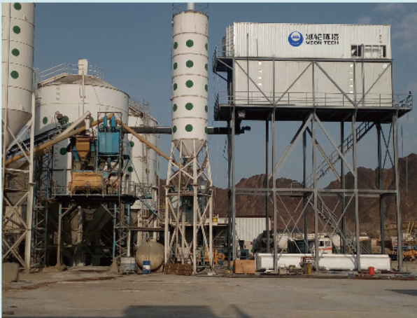
混凝土冷却自动送冰系统 2017 Automatic ice delivery system for concrete cooling 2017
